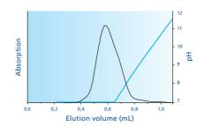
Separation of oligonucleotide from conc. ammonia after cleavage from solid support and removal of protecting groups (18-mer, Scale: 0.04 µmol, 200 µL sample volume).
