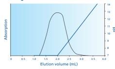
after oligo cleavage from solid support and removal of protecting groups 1.0 mL sample volume 18-mer oligonucleotide, 0.2 µmol: black line (260 nm) Ammonia, 10 M: blue line (pH) Elution with pure water **CentriPure** Gel Filtration Columns for rapid and efficient removal of small molecules from **antibodies**, **enzymes and other proteins**.
