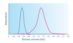
Elution profile overlay of 0.1  $\mu$ mol 5-TAMRA and 0.04  $\mu$ mol oligonucleotide (200  $\mu$ L sample volume).
