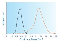
Elution profile overlay of ovalbumin (1 mg/mL) and free dye (TAMRA, 0,1  $\mu mol)$  in a 200  $\mu L$  sample volume.
