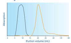
5.0 mL sample volume Ovalbumin, 5 mg: black line (280 nm) Fluorescein, 2.5 µmol: orange line (490 nm) Elution with pure water
