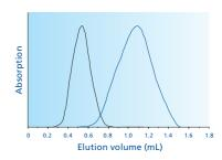
Desalting of protein solution (1 mg ovalbumin (OvA) in 1 mL 0.8 M NaCl), elution with water (200  $\mu$ L sample volume)
